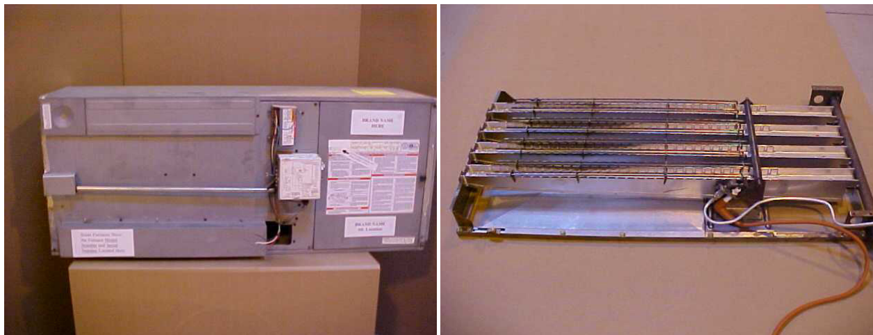
These gas-fired horizontal furnaces have steel rods (right) installed above the burners.
